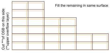
Cut of OSB (\*\*upper overflow layer) on this side
